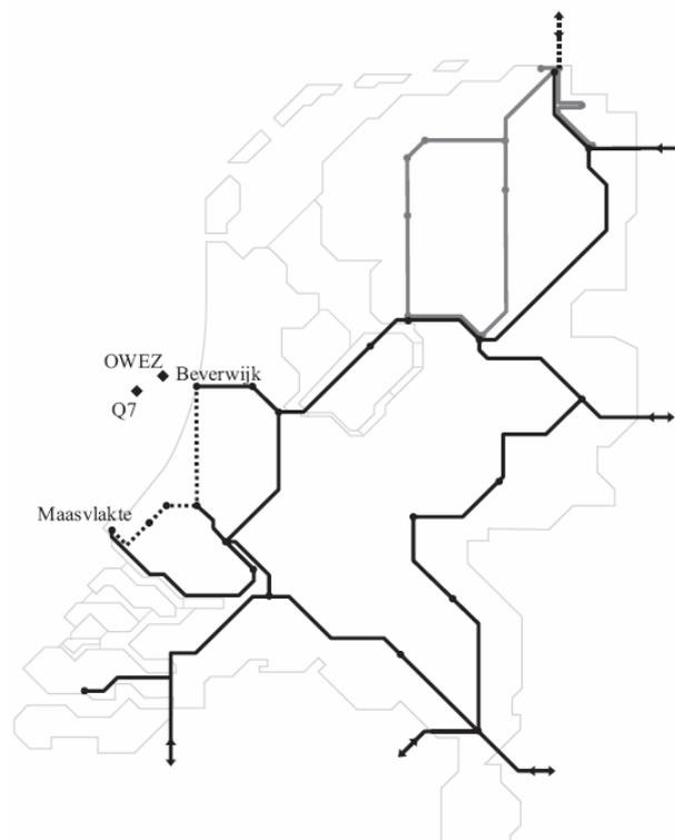
Fig. 2 A ring at the 380 kV voltage level with several radial branches
