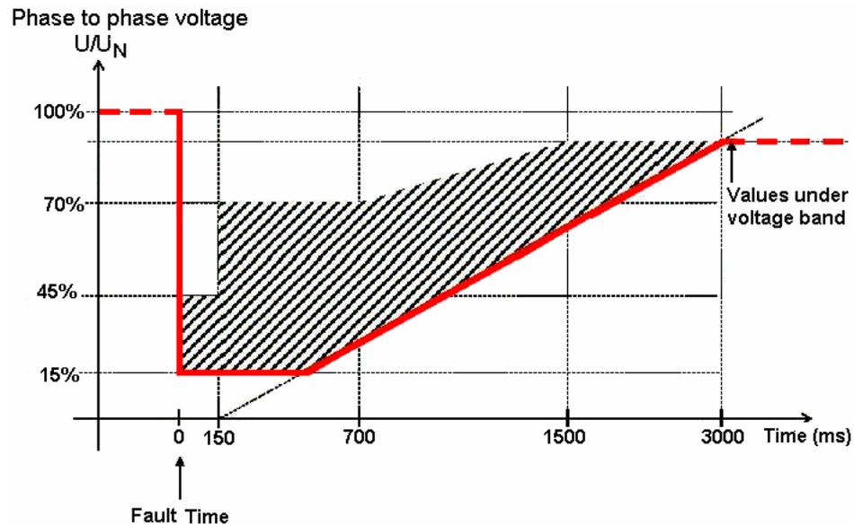
Fig-6 Failure and after failure performance of the production plants based on wind energy
