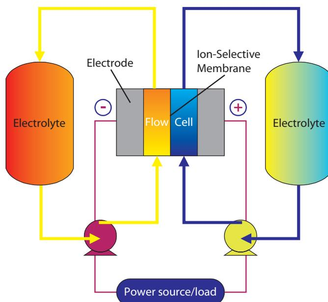
Figure 2. Schematic overview of a redox flow cell energy storage system
