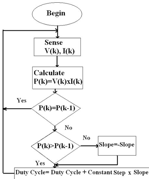
Fig. 3. Flow chart of the hill climbing MPP tracking method
