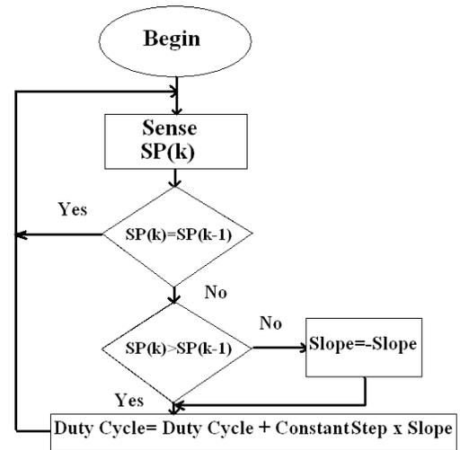
Fig.4 Flow chart of the speed control based MPP tracking method
