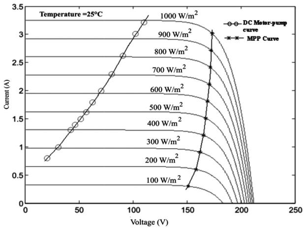
Fig. 2. DC motor-pump I-V curve on PV I-V curves for varying insolation
