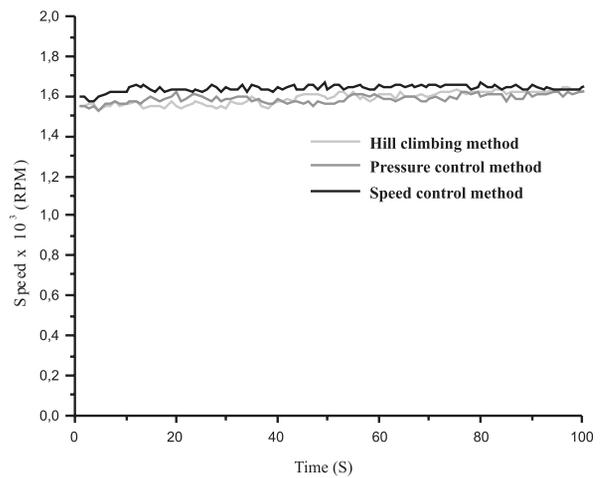
Fig. 11. Motor-pump rotation speed
