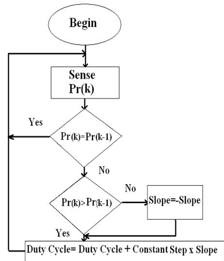
Fig. 5. Flow chart of the pressure control MPP tracking method
