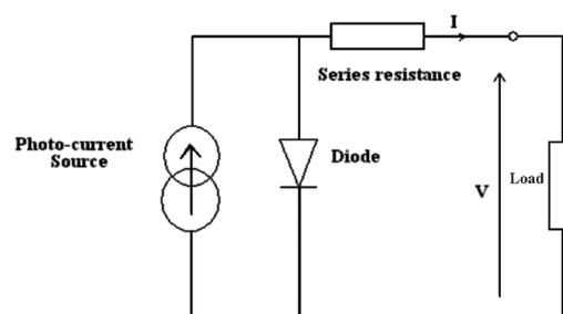
Fig. 1. Equivalent circuit of PV solar cell
