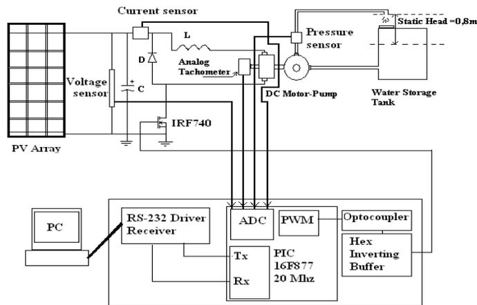
Fig. 6. Block diagram of the experimental bench
