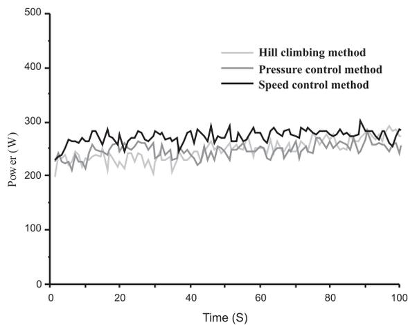
Fig. 9. PV array generated power
